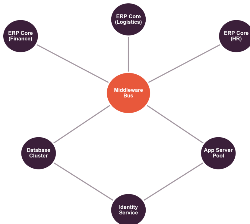
Figure 9. Illustrative Component Dependency Graph Used for Blast-Radius and Root-Cause Reasoning
